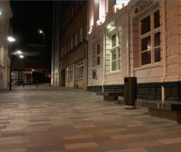
New state-of-the-art lighting installed in Nelson Street as part of the Douglas Regeneration Scheme. The lighting is low energy, high intensity LED and is the first use of this particular 75 Watt, 64 LED fitting in the British Isles – November 2011
